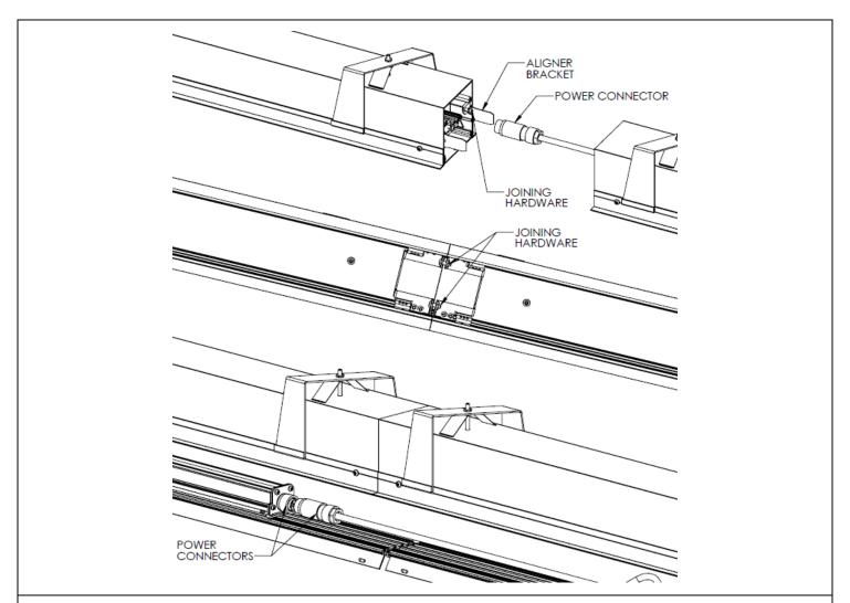
STEP 7. For continuous runs, install Start fixture first (as per steps 1-6). Do not apply power. Install joining fixture (as per steps 1-4 and step 6). Align joining fixture and slide it into place. Secure with joining hardware. And then connect power connectors together. Reinstall reflector / driver enclosure assembly and lens.
