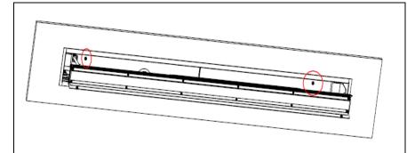
**STEP 6.** Insert fixture into drywall cutout in ceiling. Attach fixture to ceiling by turning the screws attached to the drywall brackets. The brackets will rotate over the drywall to secure the fixture. Reinstall reflector / driver enclosure assembly and lens.
