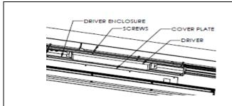
STEP 4. Remove and service driver as required. Be sure to wire correctly (both power and dimming, and the wires to LED board). Reinstall cover plate, driver enclosure to reflector assembly, ensure all wires are inside of the driver enclosure. Reinstall reflector and driver enclosure assembly to fixture. Reinstall lens.
