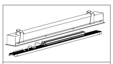
STEP 4. Lower the reflector / driver enclosure assembly
