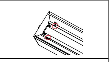
**STEP 3.** Unscrew the reflector assembly.
