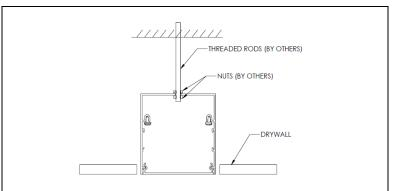
**STEP 6.** Feed threaded mounting rod (by others) through mounting locations and adjust nut to ensure fixture is parallel to drywall. Insert the fixture all the way through the opening in the ceiling. Insert the second nut (by others) through the fixture and fasten the fixture in place. Repeat with remaining mounting locations until fixture is parallel along entire length. Reinstall reflector / driver enclosure assembly and lens.
