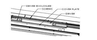
STEP 4. Remove and service driver as required. Be sure to wire correctly (both power and dimming, and the wires to LED board). Reinstall cover plate, driver enclosure to reflector assembly, ensure all wires are inside of the driver enclosure. Reinstall reflector and driver enclosure assembly to fixture. Reinstall lens.
