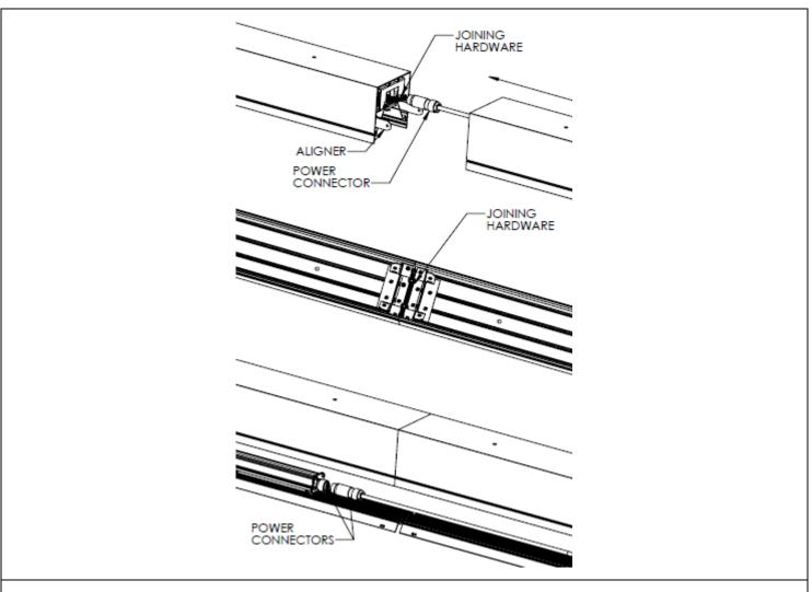
**STEP 7.** For continuous runs, install Start fixture first (as per steps 1-6). <u>Do not apply power</u>. Install joining fixture (as per steps 1-4 and step 6). Align joining fixture and slide it into place. Secure with joining hardware. And then connect power connectors together. Reinstall reflector / driver enclosure assembly and lens.
