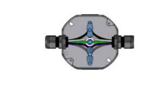
**STEP 6.** Wire fixture using waterproof wire nuts inside junction box (connector/nuts/junction box supplied by others). Refer to provided wiring diagram.
