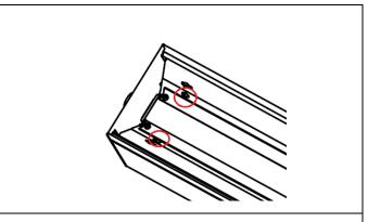
**STEP 3.** Unscrew the reflector assembly.
