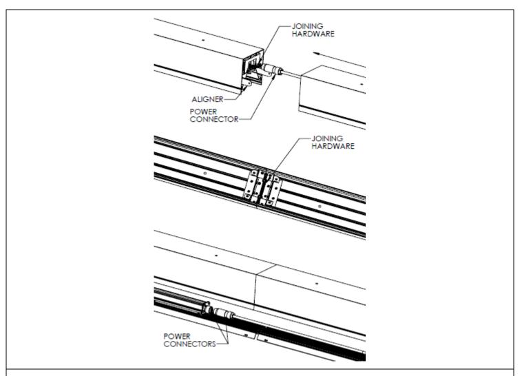
STEP 7. For continuous runs, install Start fixture first (as per steps 1-6). Do not apply power. Install joining fixture (as per steps 1-5). Align joining fixture and slide it into place. Secure with joining hardware. And then connect power connectors together. Reinstall reflector / driver enclosure assembly and lens.
