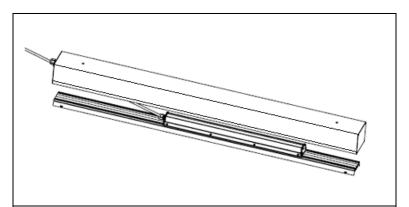
STEP 4. Lower the reflector / driver enclosure assembly, temporary hung on power cord.
