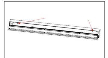
**STEP 5.** Attach fixture to ceiling using screws (supplied by others) through the holes in the extrusion. Ensure fixture is secured to a sufficiently strong structure. Reinstall reflector / driver enclosure assembly and lens.
