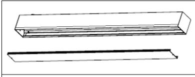
**STEP 2.** Remove the lens from the fixture.
