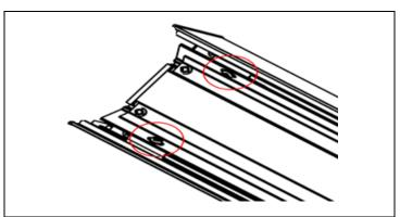
STEP 8. Remove lens from the fixture. Unscrew the reflector assembly. Lower the reflector / driver enclosure assembly, temporary hung on power cord.
