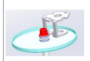
**STEP 4.** Attach both stems (and fixture) to hanger brackets.
