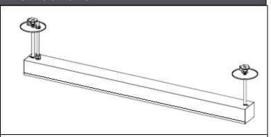
**STEP 2.** Attach stems to threaded holes at the top of the luminaire enclosure – one at each end, install power cord to the connector in the canopy.
