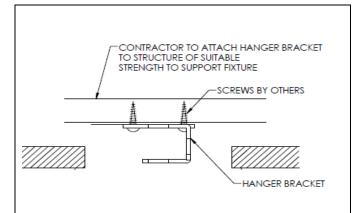
STEP 3. Remove hanger brackets from stem and attach to proper structure.
