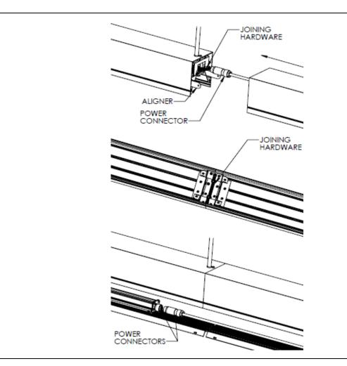
STEP 9. Align joining fixture and slide it into place. Secure with joining hardware. And then connect power connectors together. Reinstall reflector / driver enclosure assembly and lens.
