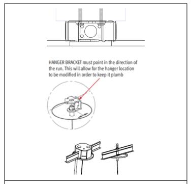
**STEP 3.** Install hanger brackets for the next fixture. Ensure bracket orientation is pointed along the run direction to allow for adjustment.
