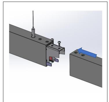
STEP 4. Make the wire connections. Align the mid/end fixture to the joint and slide it into place. Secure the joiner bracket with the provided screws (qty. 2).
